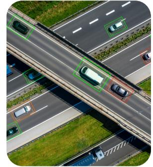
These AI sensors do not function as surveillance cameras, do not capture personally identifiable information, and do not track license plates, faces or individuals. The sensors analyze real-time traffic activity and report that data to a centralized dashboard. Intercity Transit will be able to use this data to see on-time performance and where reliability may break down, identify hot stops for operational or safety interventions, and use data to drive future planning.
