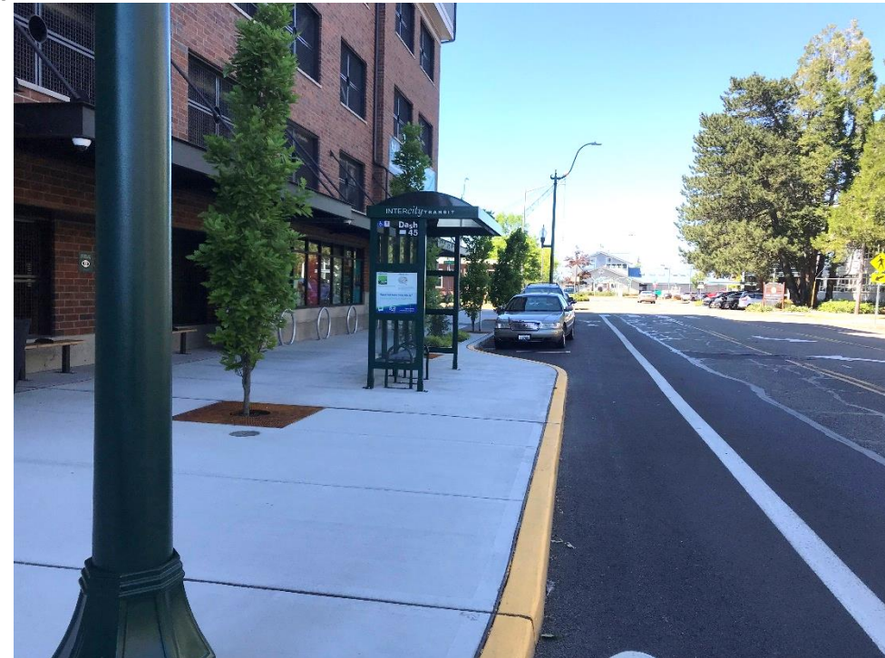
Bus stop 71 — Capitol at A [SB] — features a cantilever shelter on a bulb-out that enables an in-lane stop and all-door boarding
