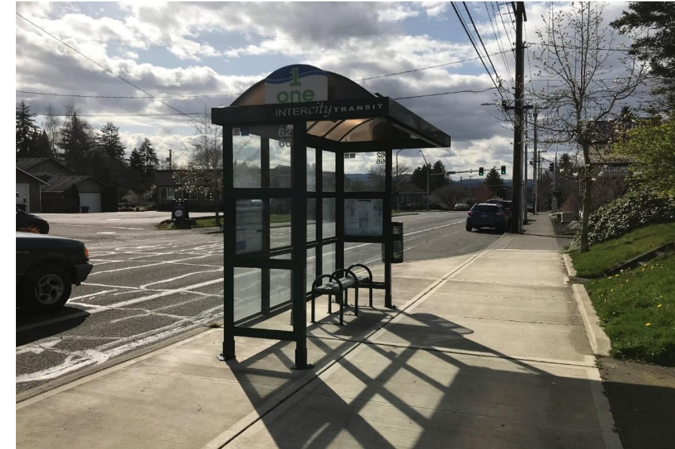
Bus stop 532 — State at Turner [WB] — features amenities including a cantilever shelter, trash can, bench, schedule, and bulbout that enables all-door boarding
